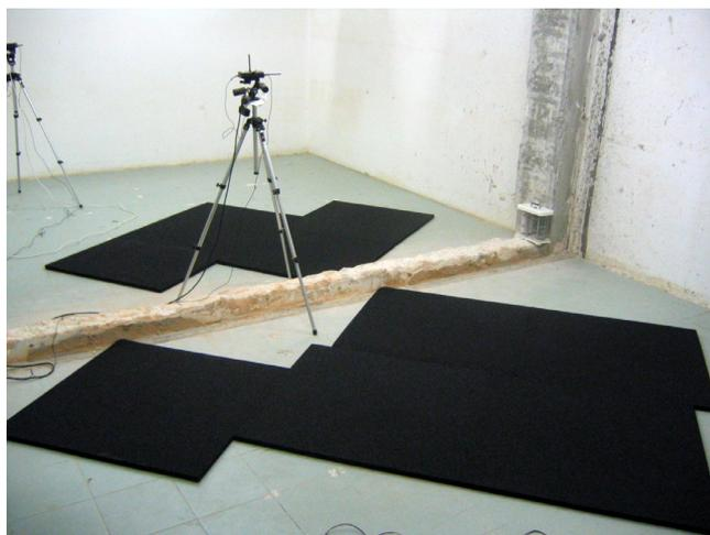
Fig. 1: View of the test specimen in the reverberation room.
